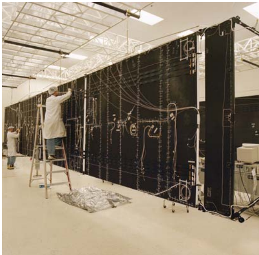
Solar Array Integration
