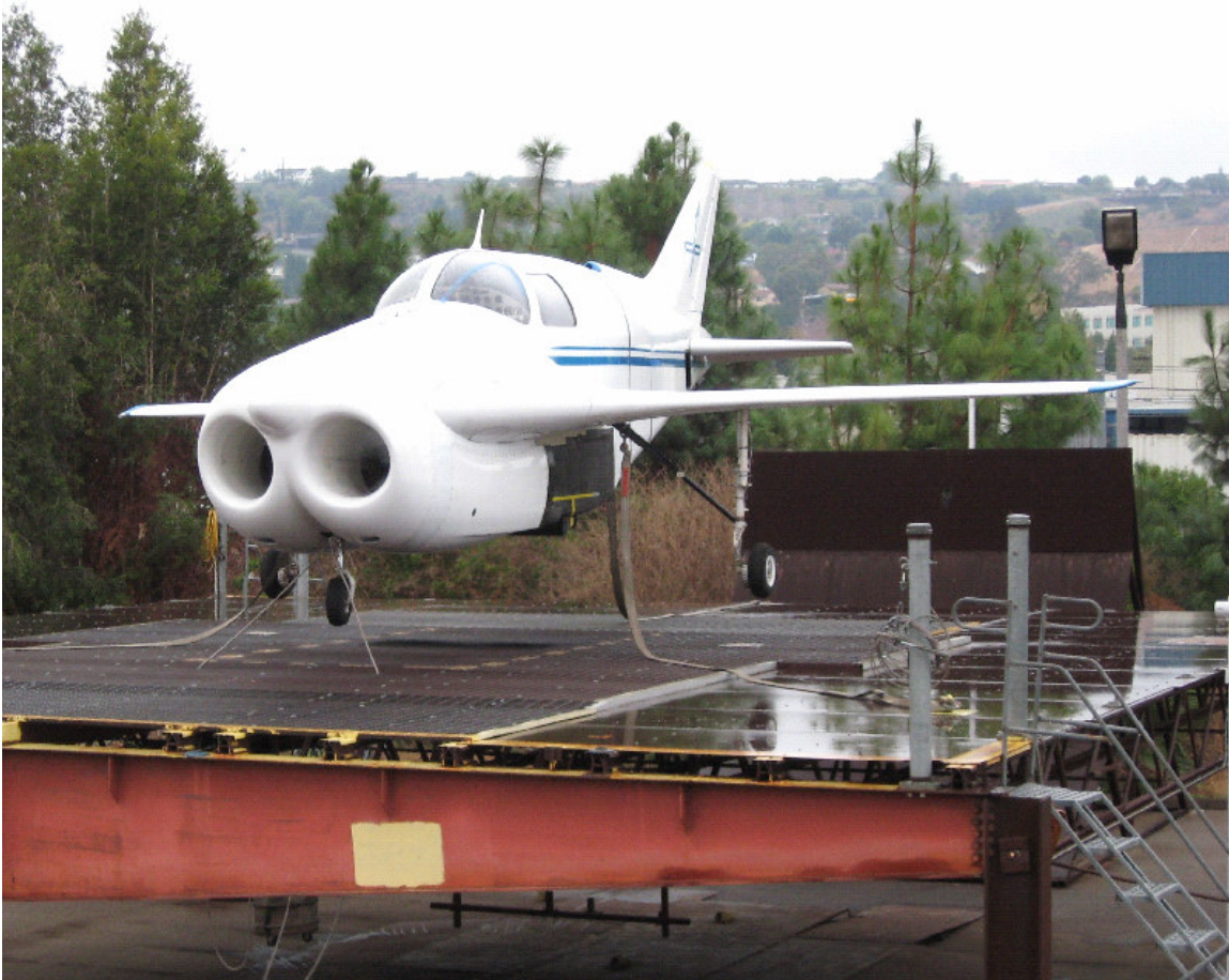
Figure 1. Still from hover video demonstrating autonomous precision hover.
